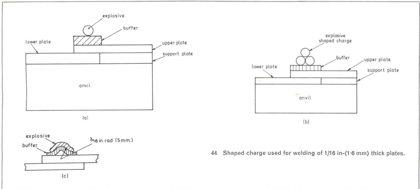
44 Shaped charge used for welding of 1/16 in-(1.6 mm) thick plates.
